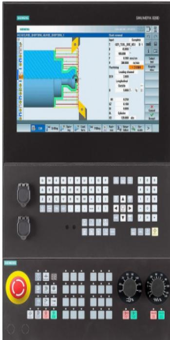
**SINUMERIK 802D BASE LINE -BT – CNC PCU210.2 BASE LINE -CNC (2 ACHSEN, 1 SPINDEL) -PLC; -HMI (10,4) -COM (PROFIBUS, RS 232), 6FC56100BB100AA1**
