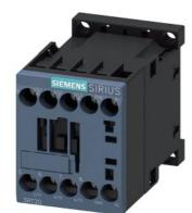
power contactor, AC-3e/AC-3, 9 A, 4 kW / 400 V, 3-pole, 380 V AC, 50/60 Hz, auxiliary contacts: 1 NC, screw terminal, size: S00
