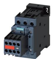
power contactor, AC-3e/AC-3, 12 A, 5.5 kW / 400 V, 3-pole, 24 V DC, with plugged-in diode combination, auxiliary contacts: 2 NO + 2 NC, screw terminal, size: S0, captive auxiliary switch
