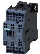
power contactor, AC-3e/AC-3, 9 A, 4 kW / 400 V, 3-pole, 24 V DC, auxiliary contacts: 1 NO + 1 NC, spring-loaded terminal, size: S0
