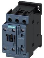
power contactor, AC-3e/AC-3, 12 A, 5.5 kW / 400 V, 3-pole, 24 V AC, 50/60 Hz, auxiliary contacts: 1 NO + 1 NC, screw terminal, size: S0
