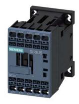
power contactor, AC-3e/AC-3, 7 A, 3 kW / 400 V, 3-pole, 400 V AC, 50/60 Hz, auxiliary contacts: 1 NC, spring-loaded terminal, size: S00  $\,$
