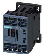
power contactor, AC-3e/AC-3, 12 A, 5.5 kW / 400 V, 3-pole, 125 V DC, auxiliary contacts: 1 NO, spring-loaded terminal, size: S00
