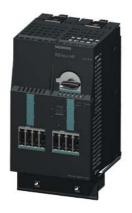
RS1E-X for ET200S High Feature reversing starter Setting range 2.4...16 A Mechanical switching Electronic protection AC-3, up to 7.5 kW / 400 V expandable for Brake control module 2DI module 2DI module Motor starter ES Circuit breaker signaling parameterizable DPV 1-capable PROFIENERGY-capable to PN
