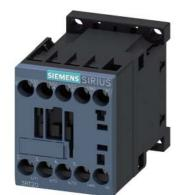
power contactor, AC-3e/AC-3, 9 A, 4 kW / 400 V, 3-pole, 120 V AC, 50/60 Hz, auxiliary contacts: 1 NO, screw terminal, size: S00
