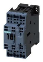
power contactor, AC-3e/AC-3, 12 A, 5.5 kW / 400 V, 3-pole, 24 V DC, auxiliary contacts: 1 NO + 1 NC, spring-loaded terminal, size: S0  $\,$
