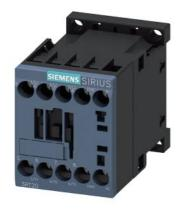
power contactor, AC-3e/AC-3, 9 A, 4 kW / 400 V, 3-pole, 24 V AC, 50/60 Hz, auxiliary contacts: 1 NC, screw terminal, size: S00
