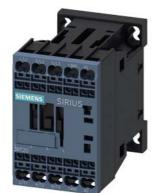
power contactor, AC-3e/AC-3, 9 A, 4 kW / 400 V, 3-pole, 110 V AC, 50 Hz / 120 V, 60 Hz, auxiliary contacts: 1 NO, spring-loaded terminal, size: S00  $\,$
