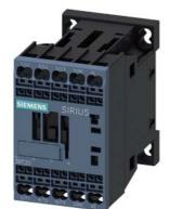
power contactor, AC-3e/AC-3, 12 A, 5.5 kW / 400 V, 3-pole, 110 V AC, 50 Hz / 120 V, 60 Hz, auxiliary contacts: 1 NC, spring-loaded terminal, size: S00  $\,$
