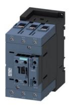
contactor AC-1, 140 A, 690 V / 40  $^{\circ}$ C, 3-pole, 220 V AC, 50/60 Hz, auxiliary contacts: 1 NO + 1 NC, main circuit: box terminal, control and auxiliary circuit: screw terminal, size: S3
