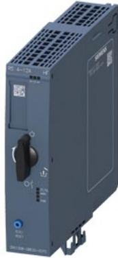
Reversing starter High Feature; Incl. fan (3RW4928-8VB00); Electronic switching; Electronic overload protection up to 5.5 kW / 400 V; Adjustment range 4.0 .. 12 A; PROFIenergy; Option: 3DI/LC module
