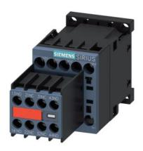
power contactor, AC-3e/AC-3, 7 A, 3 kW / 400 V, 3-pole, 24 V DC, auxiliary contacts: 2 NO + 2 NC, screw terminal, size: S00, captive auxiliary switch
