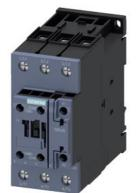
power contactor, AC-3e/AC-3, 80 A, 37 kW / 400 V, 3-pole, 83-155 V AC/DC, 50/60 Hz, with integrated varistor, auxiliary contacts: 1 NO + 1 NC, screw terminal, size: S2
