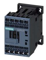
power contactor, AC-3e/AC-3, 9 A, 4 kW / 400 V, 3-pole, 125 V DC, auxiliary contacts: 1 NO, spring-loaded terminal, size: S00  $\,$
