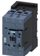
power contactor, AC-3e/AC-3, 110 A, 55 kW / 400 V, 3-pole, 230 V AC, 50 Hz, auxiliary contacts: 1 NO + 1 NC, screw terminal, size: S3  $\,$
