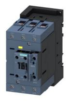
power contactor, AC-3e/AC-3, 95 A, 45 kW / 400 V, 3-pole, 21-33 V AC/DC, 50/60 Hz, with integrated varistor, auxiliary contacts: 1 NC, screw terminal, size: S3, F-PLC-IN
