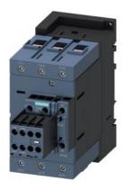
power contactor, AC-3e/AC-3, 80 A, 37 kW / 400 V, 3-pole, 110 V AC, 50 Hz, auxiliary contacts: 2 NO + 2 NC, screw terminal, size: S3, removable auxiliary switch
