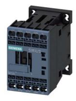
power contactor, AC-3e/AC-3, 12 A, 5.5 kW / 400 V, 3-pole, 24 V AC, 50/60 Hz, auxiliary contacts: 1 NC, spring-loaded terminal, size: S00
