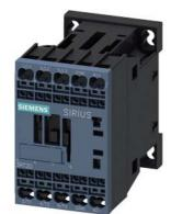
power contactor, AC-3e/AC-3, 12 A, 5.5 kW / 400 V, 3-pole, 48 V DC, with integrated diode, auxiliary contacts: 1 NC, spring-loaded terminal, size: S00  $\,$
