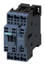
power contactor, AC-3e/AC-3, 9 A, 4 kW / 400 V, 3-pole, 200-280 V AC/DC, 50/60 Hz, with integrated varistor, auxiliary contacts: 1 NO + 1 NC, spring-loaded terminal, size: S0
