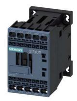
power contactor, AC-3e/AC-3, 12 A, 5.5 kW / 400 V, 3-pole, 220 V AC, 50/60 Hz, auxiliary contacts: 1 NC, spring-loaded terminal, size: S00
