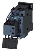
capacitor contactor, AC-6b 16.7 kVAr, / 400 V, 3-pole, 110 V AC, 50 Hz / 120 V, 60 Hz, auxiliary contacts: 1 NO + 2 NC, screw terminal, size: S0
