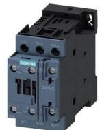
power contactor, AC-3e/AC-3, 9 A, 4 kW / 400 V, 3-pole, 48 V DC, auxiliary contacts: 1 NO + 1 NC, screw terminal, size: S0
