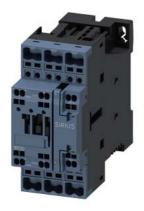
power contactor, AC-3e/AC-3, 12 A, 5.5 kW / 400 V, 3-pole, 24 V DC, auxiliary contacts: 1 NO + 1 NC, spring-loaded terminal, size: S0, communication-capable
