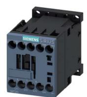
power contactor, AC-3e/AC-3, 7 A, 3 kW / 400 V, 3-pole, 24 V DC, with integrated diode, auxiliary contacts: 1 NC, screw terminal, size: S00  $\,$
