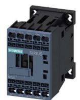
power contactor, AC-3e/AC-3, 7 A, 3 kW / 400 V, 3-pole, 110 V AC, 50 Hz / 120 V, 60 Hz, auxiliary contacts: 1 NO, spring-loaded terminal, size: S00  $\,$
