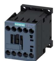
power contactor, AC-3e/AC-3, 9 A, 4 kW / 400 V, 3-pole, 230 V DC, auxiliary contacts: 1 NC, screw terminal, size: S00
