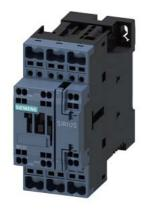
power contactor, AC-3e/AC-3, 12 A, 5.5 kW / 400 V, 3-pole, 48 V DC, auxiliary contacts: 1 NO + 1 NC, spring-loaded terminal, size: S0  $\,$
