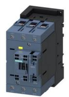
power contactor, AC-3e/AC-3, 110 A, 55 kW / 400 V, 3-pole, 175-280 V AC/DC, 50/60 Hz, with integrated varistor, auxiliary contacts: 1 NC, main circuit: screw terminal, control and auxiliary circuit: spring-loaded terminal, size: S3, F-PLC-IN
