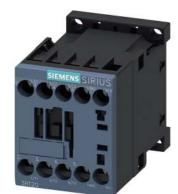
power contactor, AC-3e/AC-3, 9 A, 4 kW / 400 V, 3-pole, 72 V DC, auxiliary contacts: 1 NO, screw terminal, size: S00
