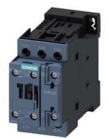
power contactor, AC-3e/AC-3, 9 A, 4 kW / 400 V, 3-pole, 21-28 V AC/DC, 50/60 Hz, with integrated varistor, auxiliary contacts: 1 NO + 1 NC, screw terminal, size: S0
