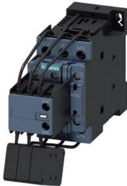
capacitor contactor, AC-6b 25 kVA<sub>r</sub>, / 400 V, 3-pole, 24 V DC, auxiliary contacts: 1 NO + 2 NC, screw terminal, size: S0
