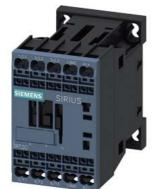
power contactor, AC-3e/AC-3, 9 A, 4 kW / 400 V, 3-pole, 125 V DC, auxiliary contacts: 1 NO, spring-loaded terminal, size: S00  $\,$
