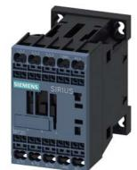
power contactor, AC-3e/AC-3, 9 A, 4 kW / 400 V, 3-pole, 220 V DC, auxiliary contacts: 1 NO, spring-loaded terminal, size: S00  $\,$
