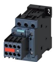
power contactor, AC-3e/AC-3, 9 A, 4 kW / 400 V, 3-pole, 24 V DC, auxiliary contacts: 2 NO + 2 NC, screw terminal, size: S0, captive auxiliary switch, no surge suppressor retrofittable
