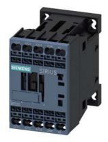
power contactor, AC-3e/AC-3, 7 A, 3 kW / 400 V, 3-pole, 230 V AC, 50/60 Hz, auxiliary contacts: 1 NC, spring-loaded terminal, size: S00  $\,$
