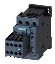
power contactor, AC-3e/AC-3, 9 A, 4 kW / 400 V, 3-pole, 230 V AC, 50/60 Hz, auxiliary contacts: 2 NO + 2 NC, screw terminal, size: S0, removable auxiliary switch
