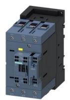
power contactor, AC-3e/AC-3, 95 A, 45 kW / 400 V, 3-pole, 175-280 V AC/DC, 50/60 Hz, with integrated varistor, auxiliary contacts: 1 NC, main circuit: screw terminal, control and auxiliary circuit: spring-loaded terminal, size: S3, F-PLC-IN
