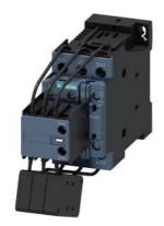
capacitor contactor, AC-6b 25 kVAr, / 400 V, 3-pole, 200-280 V AC/DC, 50/60 Hz, with integrated varistor, auxiliary contacts: 1 NO + 2 NC, screw terminal, size: S0  $\,$
