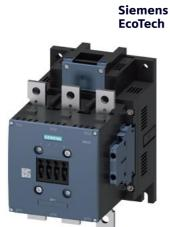
power contactor, AC-3e/AC-3 300 A, 160 kW / 400 V, AC (50-60 Hz) / DC Uc: 42-48 V 3-pole, auxiliary contacts 2 NO + 2 NC drive: conventional main circuit: busbar control and auxiliary circuit: screw terminal
