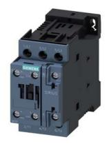
power contactor, AC-3e/AC-3, 9 A, 4 kW / 400 V, 3-pole, 21-28 V AC/DC, 50/60 Hz, with integrated varistor, auxiliary contacts: 1 NO + 1 NC, screw terminal, size: S0
