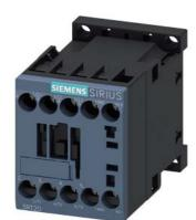
power contactor, AC-3e/AC-3, 7 A, 3 kW / 400 V, 3-pole, 24 V DC, 0.7-1.25\* Us, with integrated suppressor diode, auxiliary contacts: 1 NO, screw terminal, size: S00, suitable for PLC outputs, not expandable with auxiliary switch
