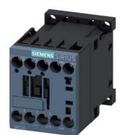
power contactor, AC-3e/AC-3, 7 A, 3 kW / 400 V, 3-pole, 24 V DC, auxiliary contacts: 1 NC, screw terminal, size: S00, communication-capable
