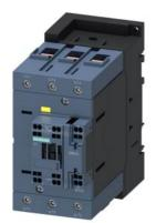
power contactor, AC-3e/AC-3, 110 A, 55 kW / 400 V, 3-pole, 83-150 V AC/DC, 50/60 Hz, with integrated varistor, auxiliary contacts: 1 NC, main circuit: screw terminal, control and auxiliary circuit: spring-loaded terminal, size: S3, F-PLC-IN
