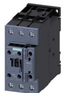
power contactor, AC-3e/AC-3, 80 A, 37 kW / 400 V, 3-pole, 230 V AC, 50/60 Hz, auxiliary contacts: 1 NO + 1 NC, screw terminal, size: S2
