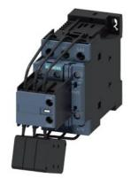
capacitor contactor, AC-6b 20 kVAr, / 400 V, 3-pole, 200-280 V AC/DC, 50/60 Hz, with integrated varistor, auxiliary contacts: 1 NO + 2 NC, screw terminal, size: S0  $\,$
